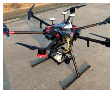
Figure 3. Unmanned aerial vehicle (UAV) hyperspectral data acquisition system
