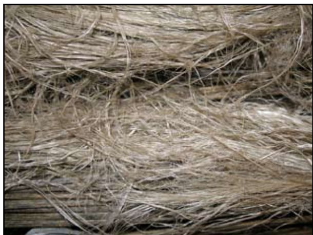
Figure 3. Dew retted hemp fibre after scutching (on the left) and after combing (on the right)
