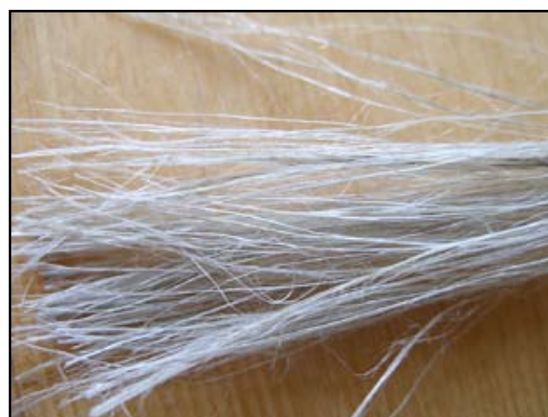
Figure 4. Water retted hemp fibre after scutching (on the left) and after combing (on the right)
