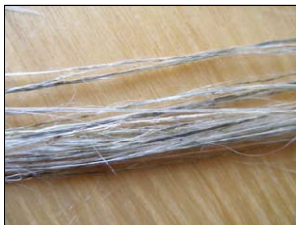
Figure 3. Dew retted hemp fibre after scutching (on the left) and after combing (on the right)
